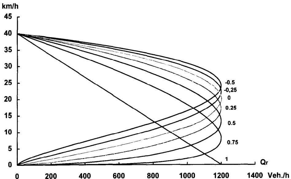
Fig. 2. Speed–flow relationships for different values of  $\gamma$  (varying between  $-0.5$  and  $1$ ).
