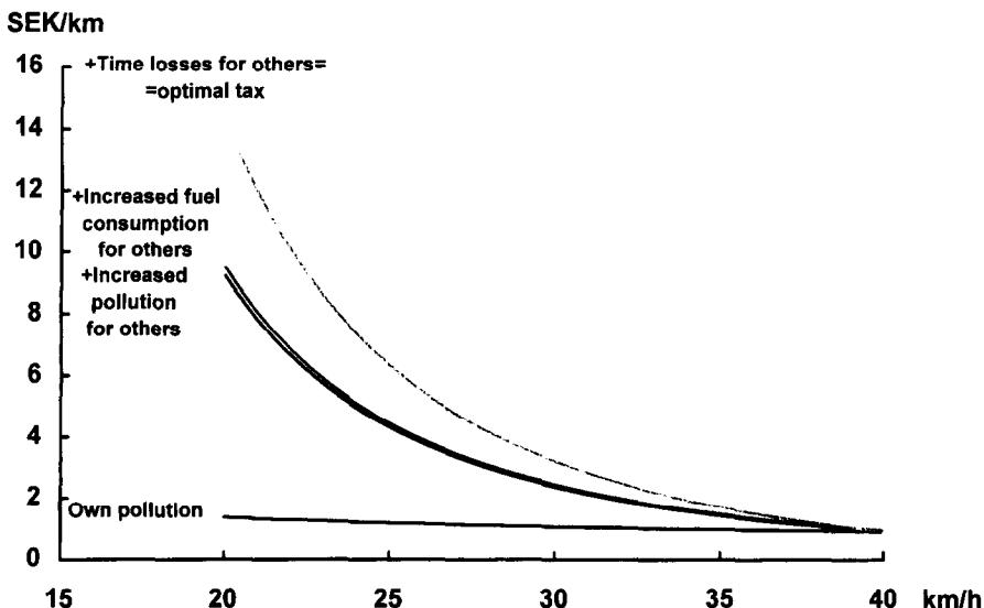
Fig. 4. Optimal road charge for a passenger car with catalytic converter with respect to the equilibrium speed divided (cumulatively) on different elements. Central street in Göteborg and unfavorable weather conditions; assumptions described in text; 10 SEK  $\approx$  1£.
