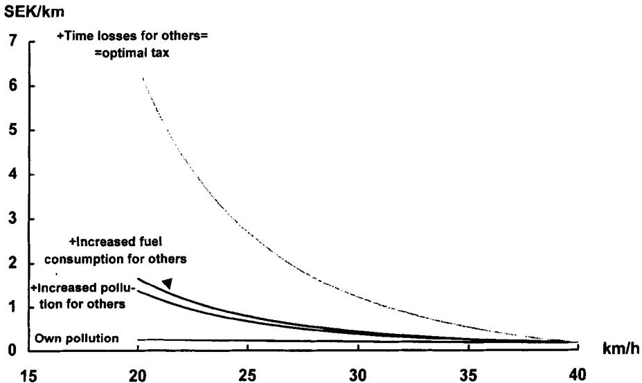
Fig. 3. Optimal road charge for a passenger car with catalytic converter with respect to the equilibrium speed divided (cumulatively) on different elements. Average conditions in Göteborg; assumptions described in text; 10 SEK  $\approx$  1£.
